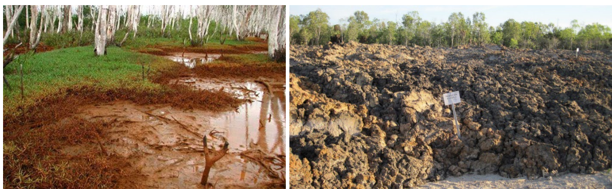
Figure 14. Acid sulphate soil in Queensland (left) and lime-treated acid sulphate soil from mangroves in Darwin (NT, Australia)
