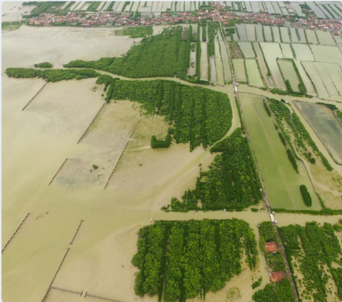
Figure 7. Permeable structures trapping mud for mangrove recovery (Source: Wetlands International, 2018).
