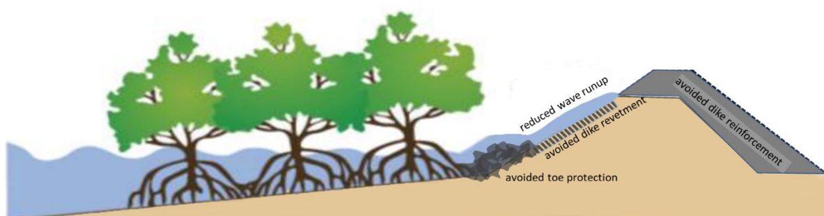
Figure 93. Schematic diagram of green-grey coastal infrastructure (adjusted from World Bank, 2017).
