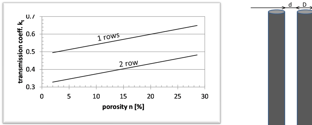
Figure 9. Indicative transmission coefficient k_t as function of fence porosity n for a single and double row fence and as a function of water depth h and wave height H_s , and definition of fence parameters (frontal view).
